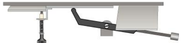
Burn Type Lever lowered (position "B"): Providing bottom air for coal burning
