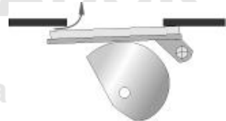
At low setting, the flap is barely open as to reduce the intake of air
