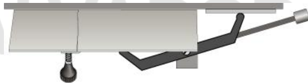
Burn Type Lever raised (position "A"): Providing top air for wood burning
