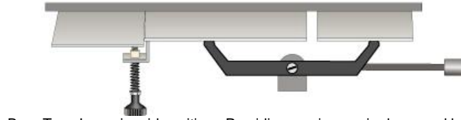
Burn Type Lever in mid position: Providing maximum air above and below grate for ignition
