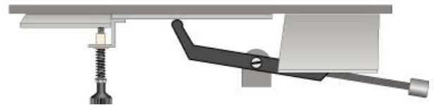
Burn Type Lever lowered (position "B"): Providing bottom air for coal burning
